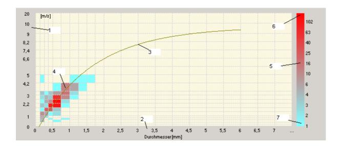
The Spectrum view provides information about the precipitation events registered in the current measuring interval. In the standard version the measuring interval is one minute. The LNM uses the distribution to determine the aggregate state and the amount of precipitation.
